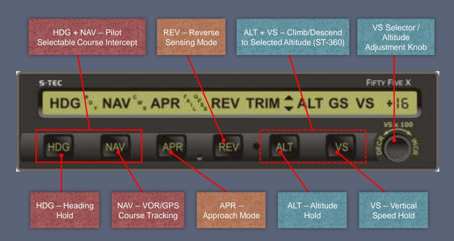
One of the lateral modes (HDG, NAV, APR/REV) must be engaged before any vertical mode (ALT, VS, GS) can be engaged
