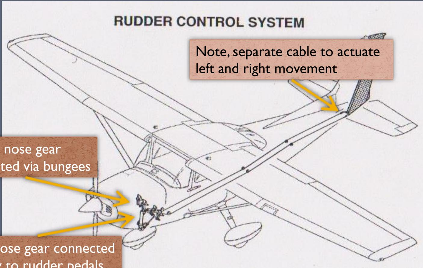
Note, separate cable to actuate left and right movement
