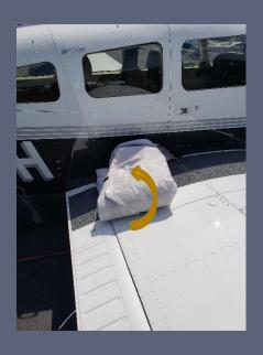
6) Fold the cover in half one more time before placing in the baggage compartment (it fits well on the hat shelf)
