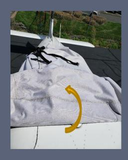
3) Fold the cover the short way from the front of the aircraft to the rear (~5 folds work well)
