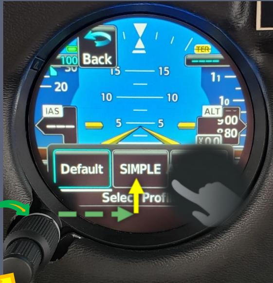
4) Scroll to the desired profile, and tap on it or press the inner knob
