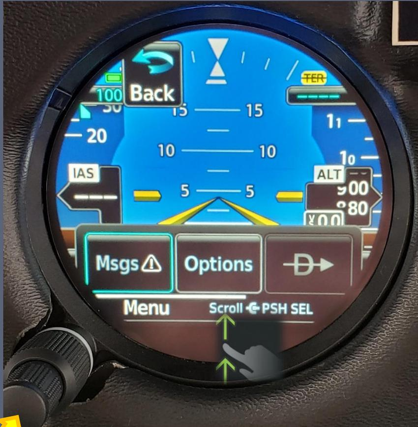
1) Press & hold the inner knob, or swipe from the bottom of the screen upwards to open the menu.
