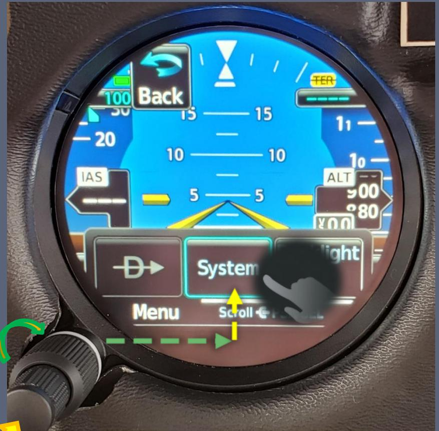
2) Scroll to the right with the outer (big) knob to “System”, and tap on it or press the inner knob.
