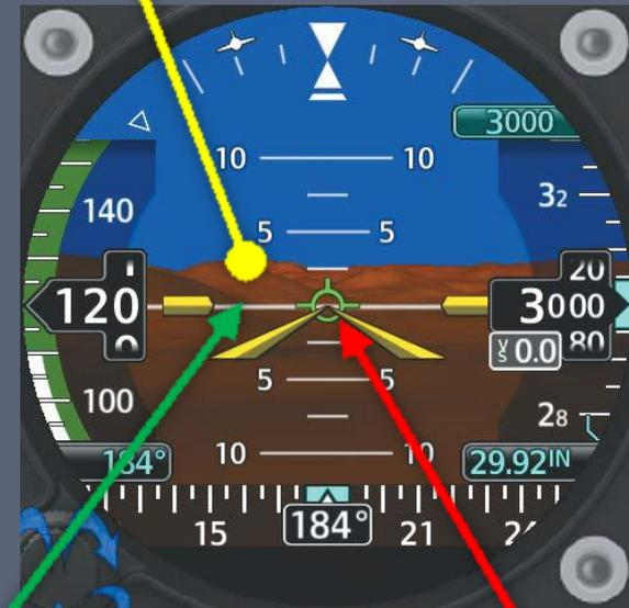
The main difference with SVT is the addition of artificial terrain and the flight path marker
