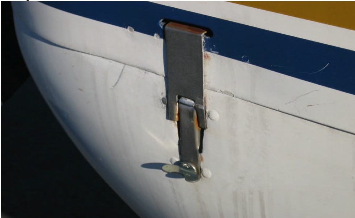
Correct fastening of Cowl Latch—the upper end of the pivoting part of the latch mechanism must engage under the downward-bent metal lip on the lower cowling.
